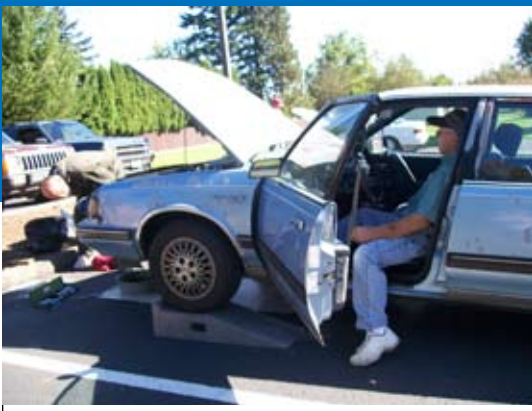
Chris Swoverland removes the oil drain pan from under a neighbor's car as his father, Pete Swoverland, prepares to back the car off the ramps.
