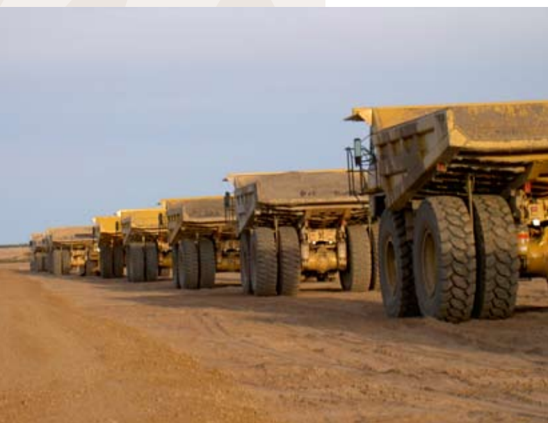
Caterpillar 777 haul trucks remove waste material above an oil sands excavation site.
